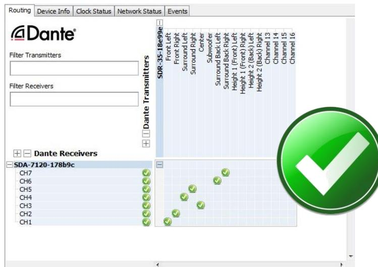
**Important Note:** Configurations are stored in DANTE devices – not in Dante Controller. At power up and/or reconnection, all subscriptions are re-established. Subscriptions are made in real time. Saving the configuration in DANTE Controller is not required.
