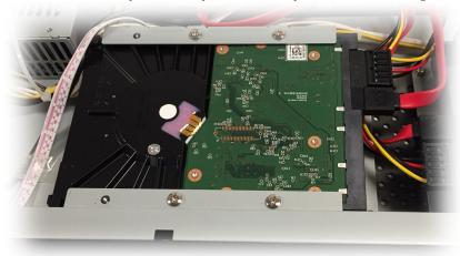
first disconnect the SATA and power cables from that hard drive.
