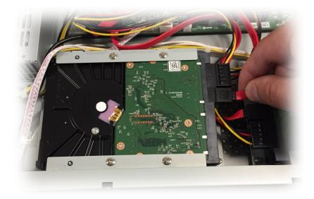
Insert four screws (as shown below) to hold the hard drive in place.
